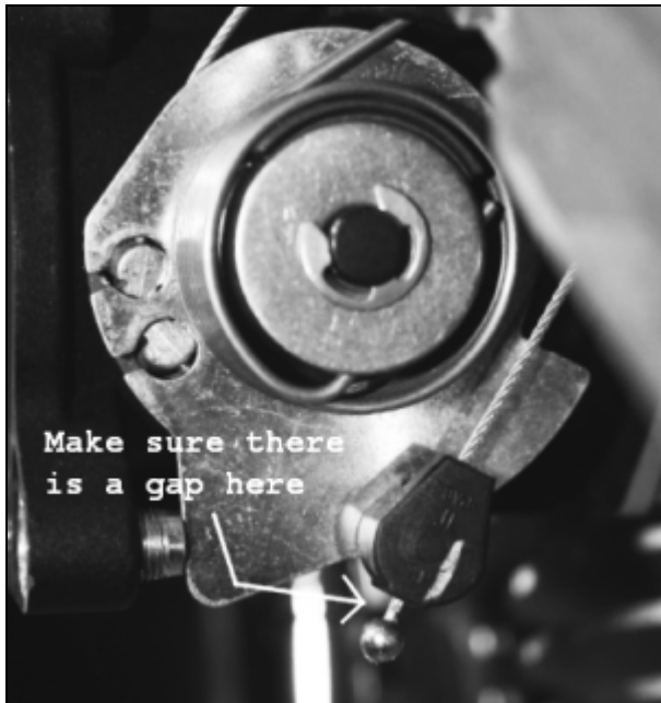
Figure 12. Check for Slack in Cable
