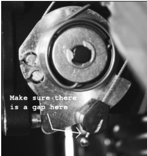
Figure 12. Check for Slack in Cable
