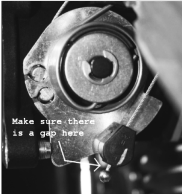
Figure 12. Check for Slack in Cable
