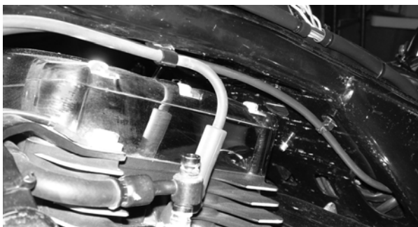
Figure 3. Cruise Control Cable Routing
