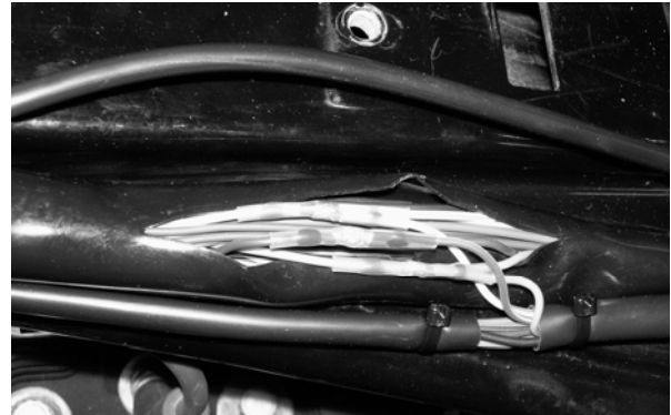
Figure 6. Splice Wires into Main Harness.
