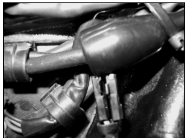
Figure 4. Throttle Roll-off Switch
