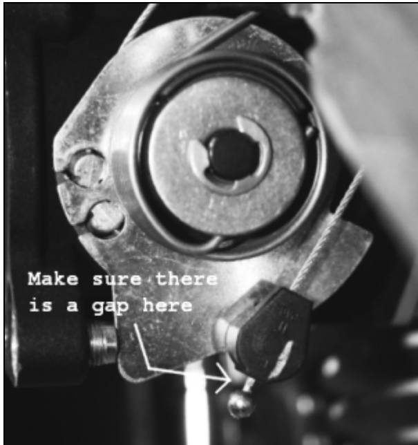
Figure 12. Check for Slack in Cable
